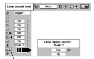
Move the pointer to Lamp counter reset and then press SELECT button. The message "Lamp replace counter reset?" is displayed.
